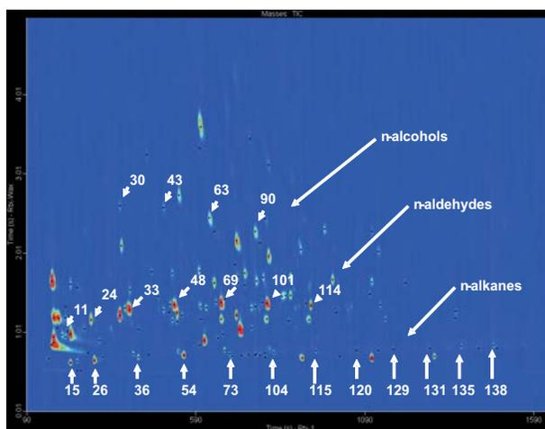
Figure 1. GCxGC chromatogram (contour plot) of SPME analysis of a \$1 bill. The total ion count (TIC) is shown with red being the most intense color. More than 300 compounds were detected by the TOFMS with a run time of less than 30 minutes. The numbered compounds, representing n-alkanes, n-aldehydes, and n-alcohols were identified by ChromaTOF software and are listed in Table 1.
